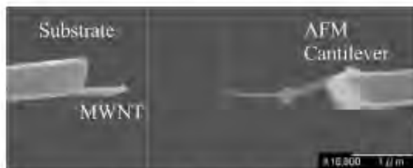
(b) After Destructive Pulling
