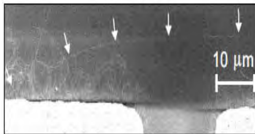
Fig. 2. SEM image of a single walled carbon nanotube. Length is 60 μm.
