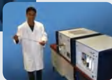
CS analyzer with high-temperature tube furnace
