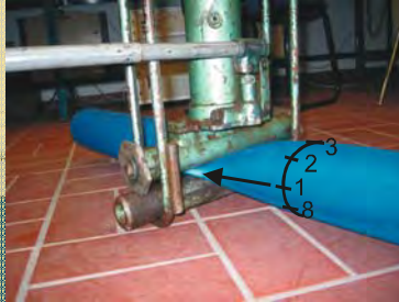
deformed PE pipe and measurement positions
