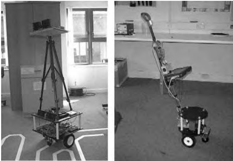
Figure 19.9: Examples of mobile robots employed for indoor channel measurements
