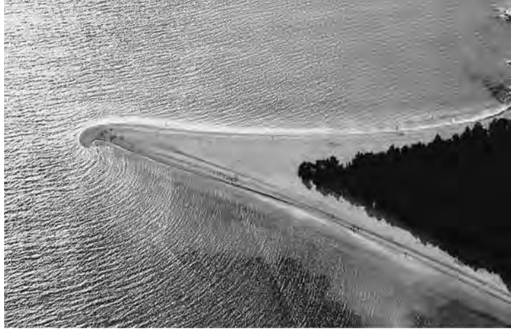
Figure 3.14: Knife-edge diffraction of waves on the sea surface
