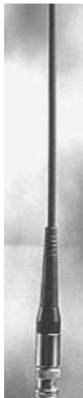
Figure 15.5: Sleeve dipole construction principles and a practical example (Reproduced by permission of Jaybeam Wireless )
